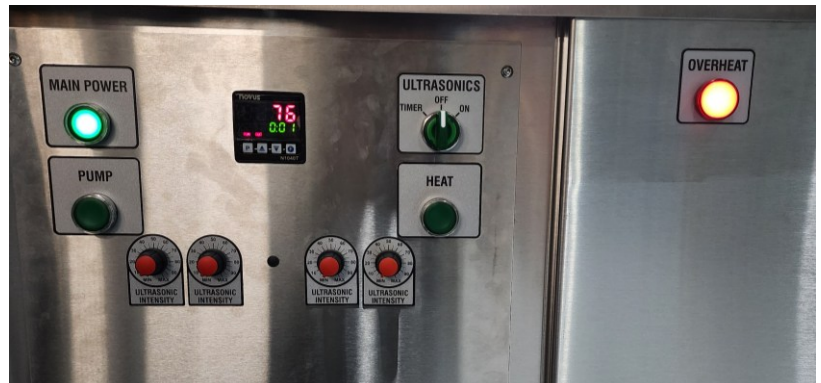
Figure 2: Over Temp Triggered
